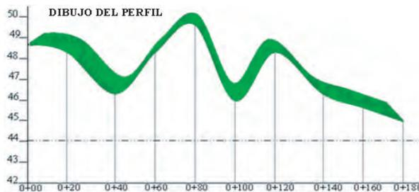
Escala Horizontal: 1/1000, Escala Vertical: 1/100; EH: 1cm = 10m, EV: 1cm = 1m.
